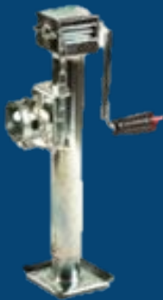
Parking Jack Capacity: 900kg Stroke: 250mm Extended: 430mm 324-PJ017
