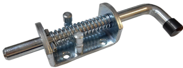
Medium Spring Bolt Pin size: 12mm Body size: 74x40mm Steel: SB12M S/Steel: SB12-SS
